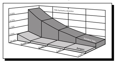
The Harmonics graph illustrates the advantage of using the Aeroport over a conventional tube. The human ear can sense .1% distortion. A standard tube can reach that amount with only 10 watts of input where as the Aeroport reaches only .05% distortion with 50 Watts of input. The end result? You can apply more input power with less distortion or use a smaller diameter Aeroport in place of a standard tube.
